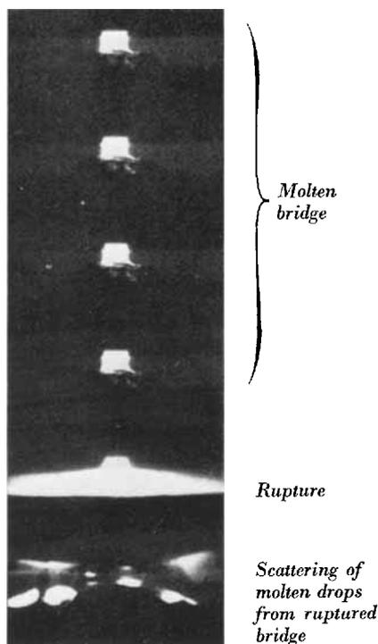
*Disruption of molten bridge between separating platinum contacts in helium, breaking a direct current of 100 amperes at 6 volts. (Capacitance 4 F, inductance 0.06 H). 9000 frames per second,  $\times 26$ . (Courtesy of Dr F. Llewellyn-Jones.)*
