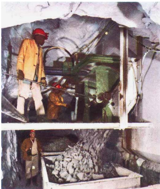
*From the working face the platinum ore is loaded into small panel cars, tipped into a central gulley and then scraped into a stope box. Here it is being transferred from the stope box into haulage cars for conveyance to the surface*
