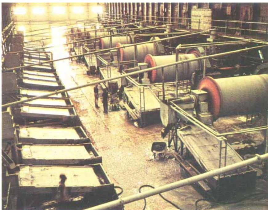
*After preliminary crushing the ore is fed to the primary and secondary ball milling sections*
