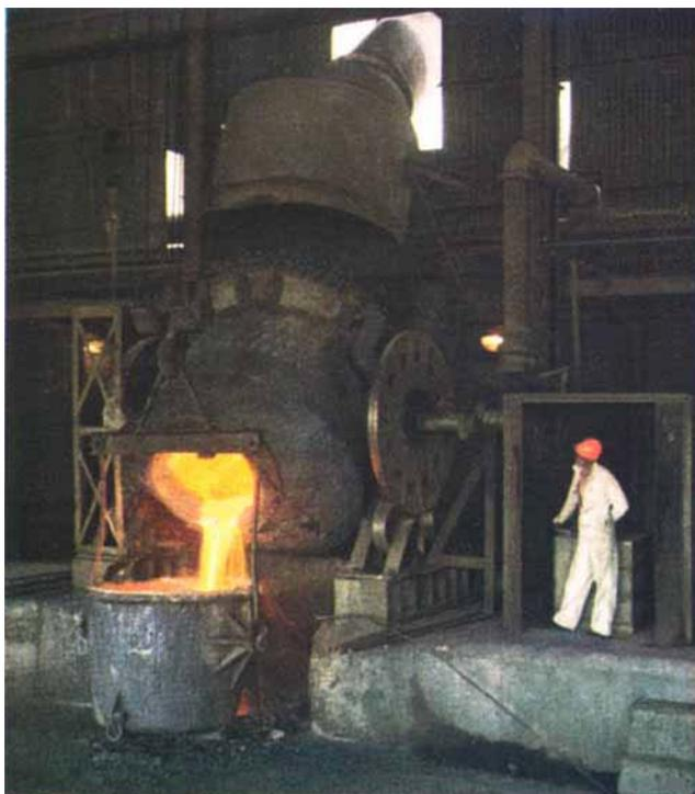
*Pouring blown matte from one of the converters. After casting and breaking up, the matte is shipped to Johnson Matthey for the extraction of copper, nickel and the six platinum metals*
