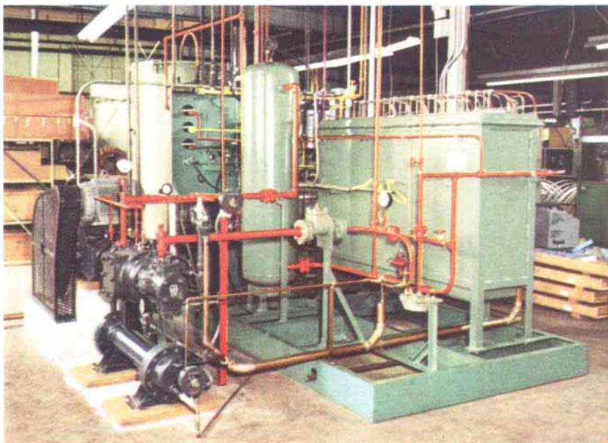
*The rear view of the hydrogen diffusion system shows the ammonia dissociator in the background and the diffusion cell heating chamber at the right*
