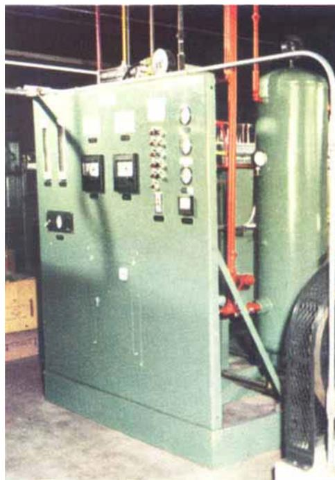
*The main control panel of the Matthey Bishop 1500 cubic feet per hour hydrogen diffusion system installed at Kreislser Industrial Corporation*
