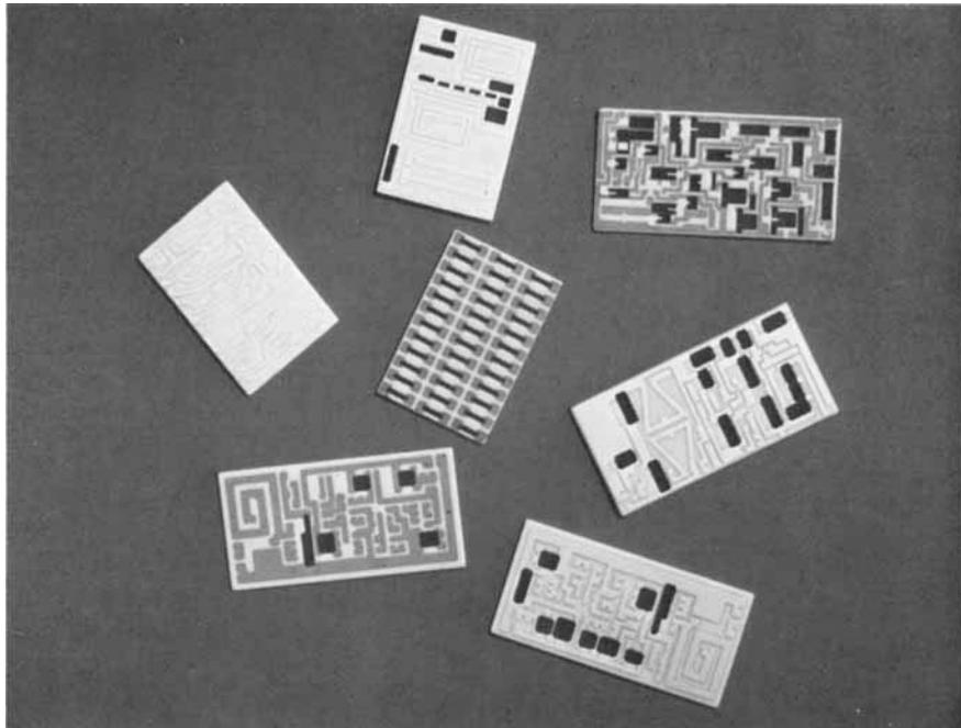
*Fig. 1 Thick film circuits on alumina substrates in the course of preparation, showing a few of the wide range of circuit configurations that can be produced by the screen printing and firing technique. The dark areas are ruthenium-based resistors interconnected with various noble metal conductors*
