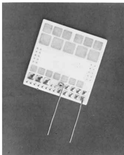
*Fig. 3 A test pattern of conductor areas used in assessing the solderability and adhesion of fired inks*
