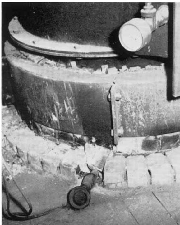
*A Pallador II thermocouple installed at the base of a recuperator at Llanelli Steel Co.*
