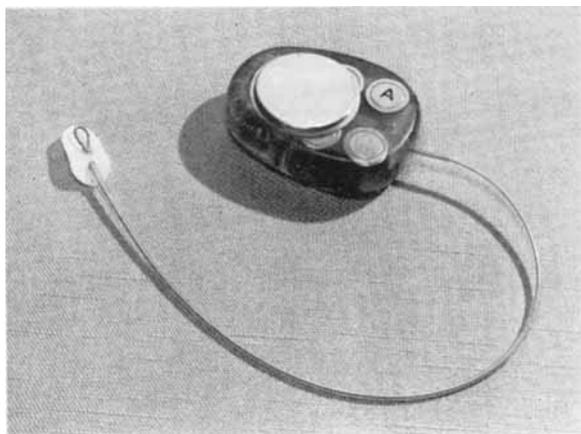
Prosthetic implants in the human body must be constructed from materials which resist the corrosive action of body fluids. Devices Implants Limited has developed a fixed-rate heart pacemaker suitable for either transvenous or transthoracic pacing. It rests in a subcutaneous pocket.
