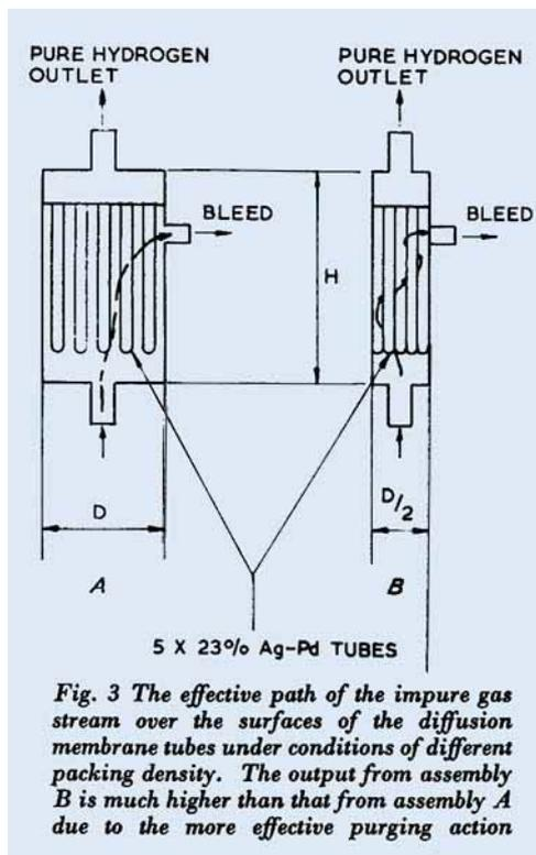
are best satisfied by the use of small diameter thin-walled tubes. These not only provide a large surface area for diffusion but they can be economically produced by conventional tube drawing techniques.
