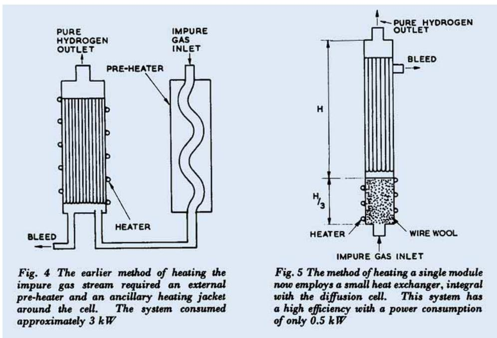
*Fig. 4 The earlier method of heating the impure gas stream required an external pre-heater and an ancillary heating jacket around the cell. The system consumed approximately 3 kW*
