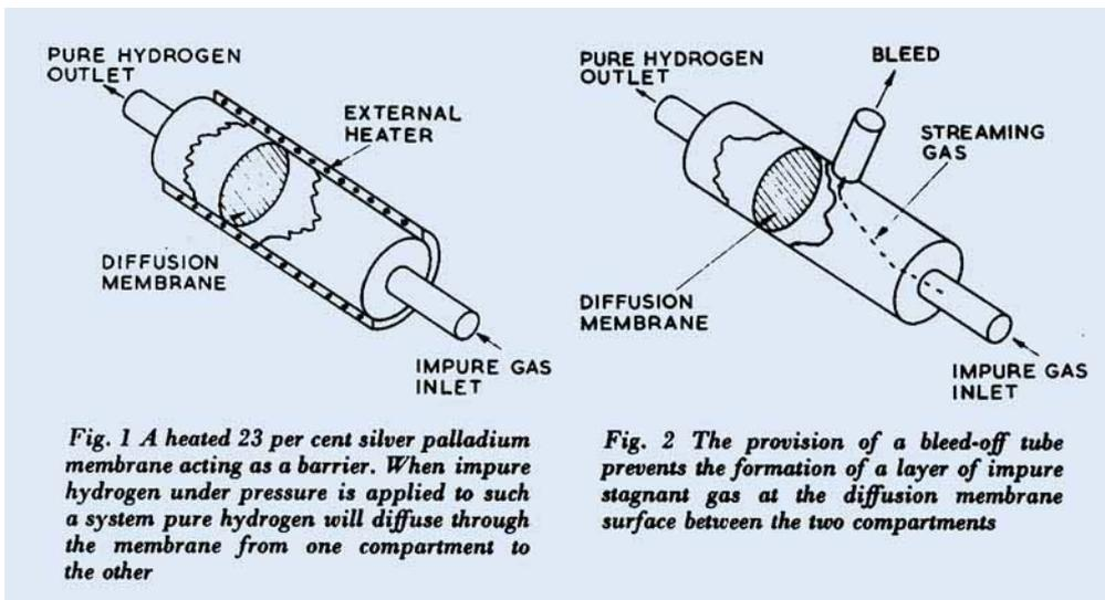
In an assembly of the type shown in Fig. 1, where a heated 23 per cent silver-palladium alloy membrane acts as a barrier between the two compartments, pure hydrogen will diffuse through the membrane from one compartment to the other.
