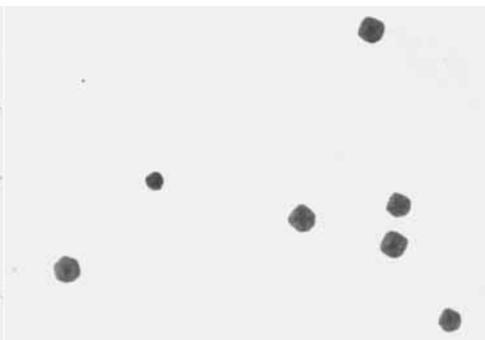
Fig. 12 Graphite spheroids precipitated from 0.25% carbon-palladium alloy by ageing at 800°C for 1 hour.  $\times 75$
