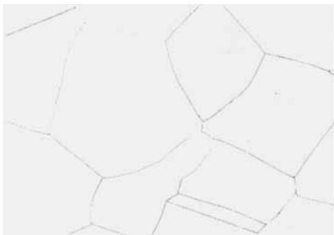
Fig. 11 Palladium containing 0.25% of carbon in solid solution quenched from 1200°C.  $\times 75$
