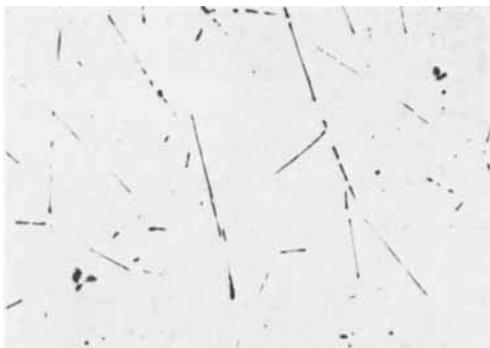
Fig. 14 As cast carbon-platinum ingot after heating in air for 90 hours at 1400°C.  $\times 75$
