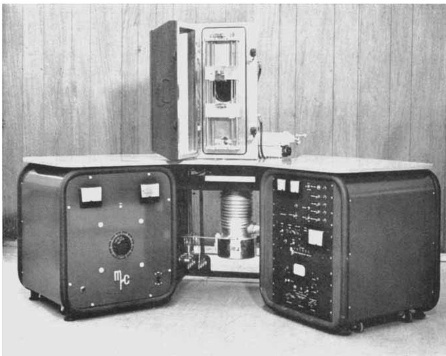
Fig. 3 An electron beam float-zone refiner. The platinum rod is given three vertical zone-refining passes at a zoning speed of three inches per hour
