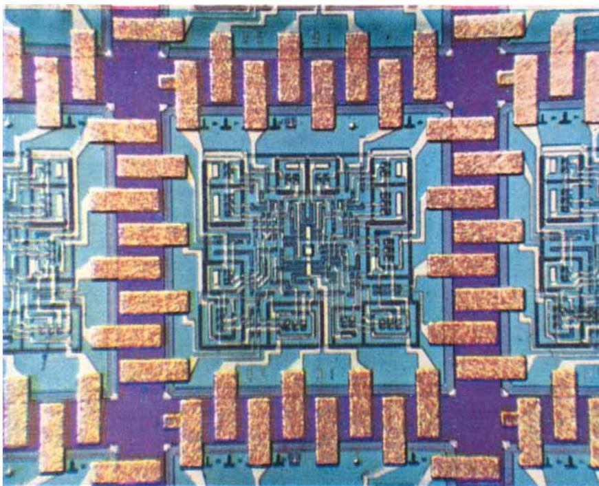
*Fig. 1 A completed beam-lead monolithic integrated circuit. Each polished silicon wafer 150–200 $\mu$  thick can hold of the order of 600 integrated circuits. (Courtesy of Western Electric Eng., December 1967.)*
