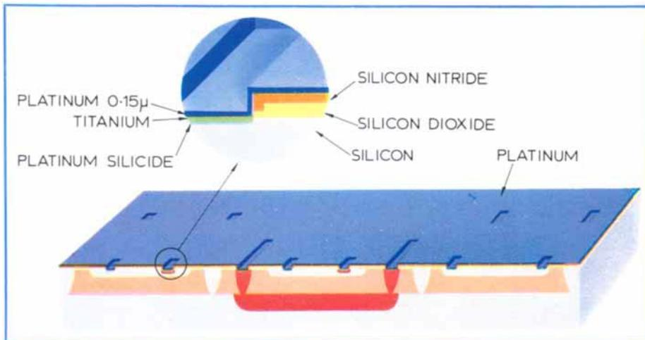
Fig. 2 Cross section of part of a crystalline silicon wafer after deposition of platinum. Typically there are between 100 and 200 stages in the complete process of integrated circuit manufacture. (Courtesy of Western Electric Eng., December 1967.)
