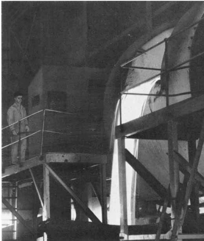
*The copper-nickel-iron matte containing the platinum metals is tapped from the electric furnace, transferred to Pierce-Smith converters and blown to a higher grade matte. Here the converter matte is being poured into moulds. After cooling and breaking up it is passed either to Johnson Matthey or to Matte Smelters for the extraction of copper, nickel and the six platinum metals*
