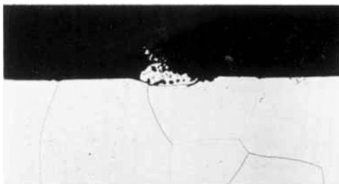
Fig. 4 Local areas of reaction between pure platinum and the coarse alumina particles in contact with it after 72 hours at 1475°C in vacuum.  $\times 150$
