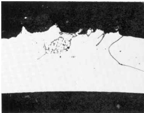
*Fig. 2 Fused zone of platinum thermocouple limb after failure in contact with fine "Purox" alumina powder after 8½ hours at 1475°C under a gettered argon atmosphere. ×150*
