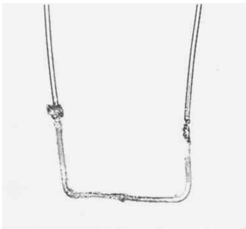
Fig. 11 Pt:13 per cent Rh-Pt thermocouple after 113 hours at 1700°C in thoria in vacuum.  $\times 2.5$
