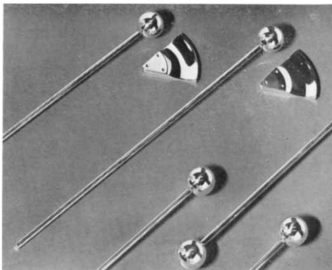
At the Radio and Space Research Station, Slough, rocket payloads are built for investigation of the production and density of ionisation in the D-region of the ionosphere at altitudes between 65 and 100 kilometres. Several different experiments are combined in each rocket flight, and one of these is a spherical Langmuir probe for measurement of electron density.
