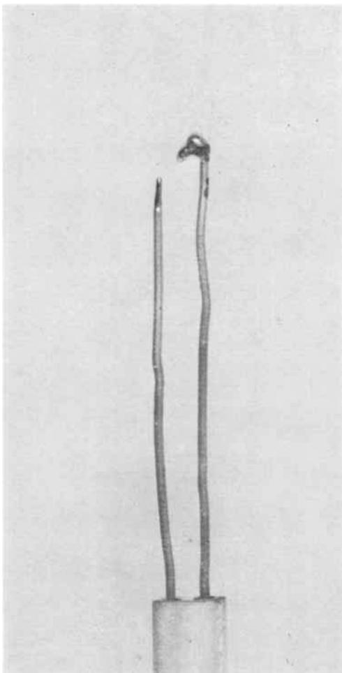
*Fig. 2 Fusion at the hot junction of a platinum : 13 per cent rhodium-platinum thermocouple sheathed with alumina and inserted vertically upwards into a furnace containing an atmosphere of dissociated ammonia at 1450°C. × 25*
