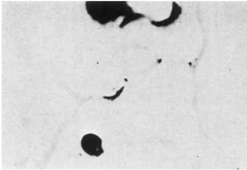
*Fig. 6 Networks of the platinum-platinum silicide eutectic formed in the vicinity of a siliceous inclusion, encapsulated in rhodium-platinum, on heating in air.* × 1500
