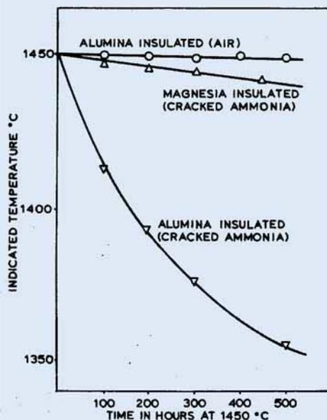
Fig. 1 The thermoelectric stabilities of platinum:13 per cent rhodium-platinum thermocouples insulated with alumina in air and dissociated ammonia, and with magnesia in dissociated ammonia. The true hot junction temperature in each case was 1450°C.
