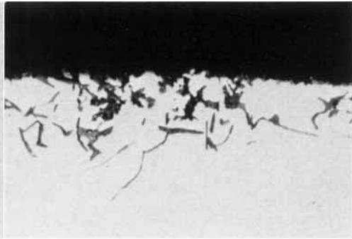
*Fig. 7 Subsurface rhodium oxide in a 13 per cent rhodium-platinum thermocouple wire operated in air for approximately 5 years at about 400°C.* × 750
