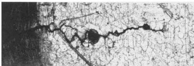
*Fig. 5 A microsection taken through a defect of the type illustrated in Fig. 4 showing the fused area resulting from reaction between a refractory particle and the rhodium-platinum alloy. × 50*
