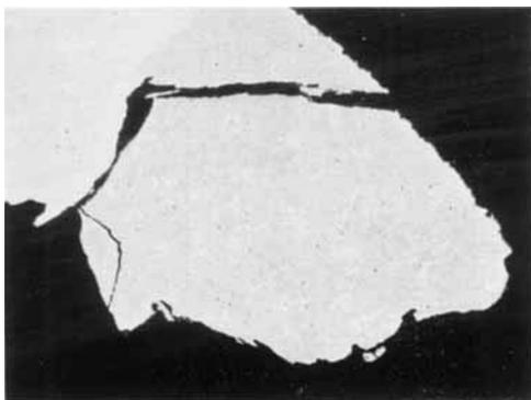
*Fig. 3 The microstructure of the fused zone on the failed thermocouple illustrated in Fig. 3. × 200*
