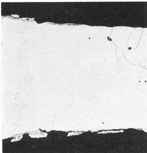
Fig. 9 Traces of the Pt<sub>3</sub>Al intermetallic compound formed locally on the surface of a platinum thermocouple wire operated in a vacuum furnace for 100 hours at 1400°C. ×150
