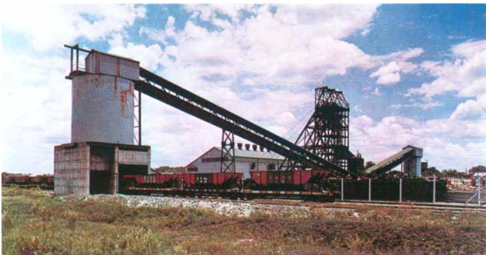
*A train load of platinum ore is transported from one of the nine vertical shafts at Rustenburg to the nearby mill and smelter. Every working day some 20,000 tons of ore are brought to the surface*
