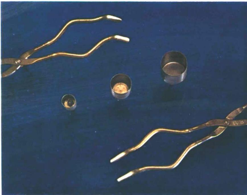
as a seed holder in a molten calcium germanate bath, and a copper thermal E.M.F. probe have been heavily coated with platinum or iridium for corrosion resistance. Objects were electroformed of platinum or iridium using suitable mandrel metals.
