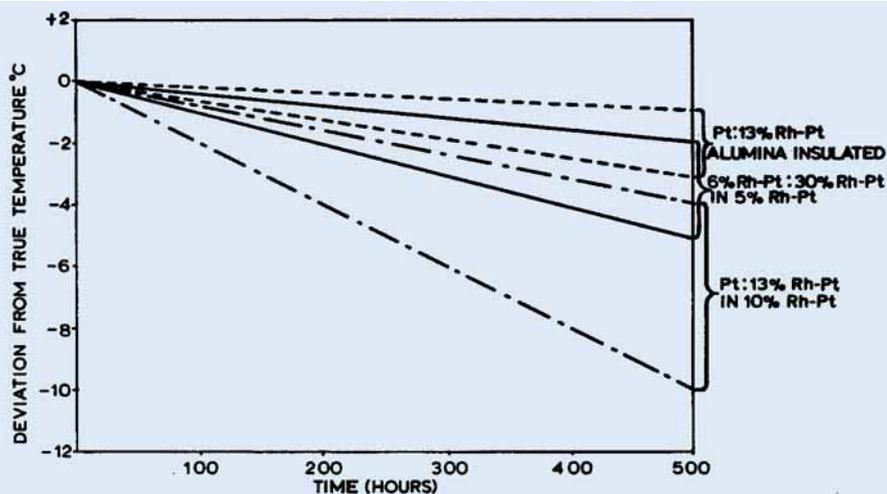
Fig. 9 Drift characteristics of argon-filled magnesia-insulated metal-sheathed thermocouples compared to those of alumina-insulated alumina-sheathed thermocouples at 1450°C in air
