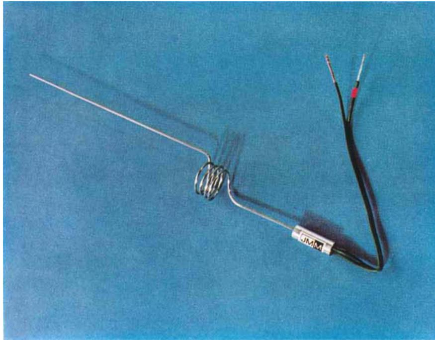
*Metal-sheathed platinum alloy thermocouples possess high stability over long periods when residual air is removed from the sheath and is replaced by an inert gas before hermetic sealing. Versatile instruments of this type are produced by Johnson Matthey Metals*
