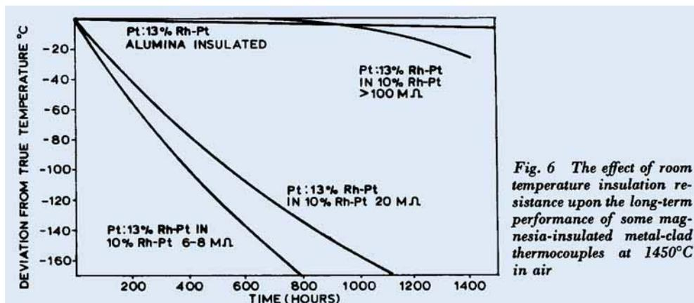
Fig. 6 The effect of room temperature insulation resistance upon the long-term performance of some magnesia-insulated metal-clad thermocouples at 1450°C in air
