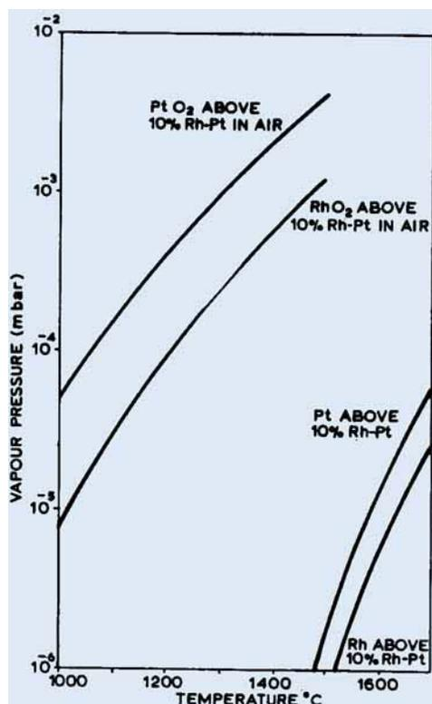
Fig. 3 The vapour pressures of rhodium, platinum, and their oxides above a 10 per cent rhodium-platinum surface in air as a function of temperature
