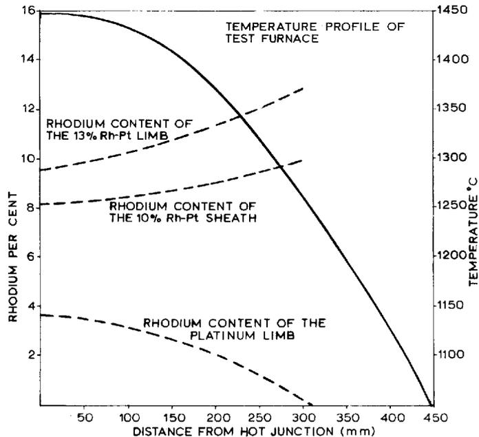
*Fig. 1 Rhodium distribution in the sheath and limbs of a platinum : 13 per cent rhodium-platinum thermocouple clad with 10 per cent rhodium-platinum after immersion for 1400 hours at a hot junction temperature of 1450°C*
