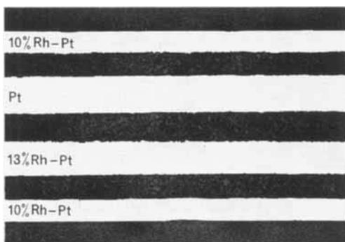
Fig. 2 A metallographic section taken through the heated zone of an unstable metal clad rhodium-platinum thermocouple after long-term exposure at 1450°C in air. The sheath and positive limb show clear signs of the erosion resulting from metal losses through the vapour phase
