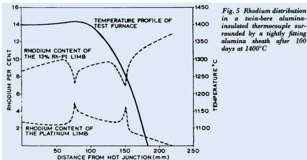
Fig. 5 Rhodium distribution in a twin-bore alumina-insulated thermocouple surrounded by a tightly fitting alumina sheath after 100 days at 1400°C
