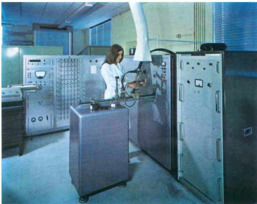
*This modern direct reading spectrograph can detect impurity levels for many elements down to less than 1 part per million and can record these levels for 42 elements in a single operation*
