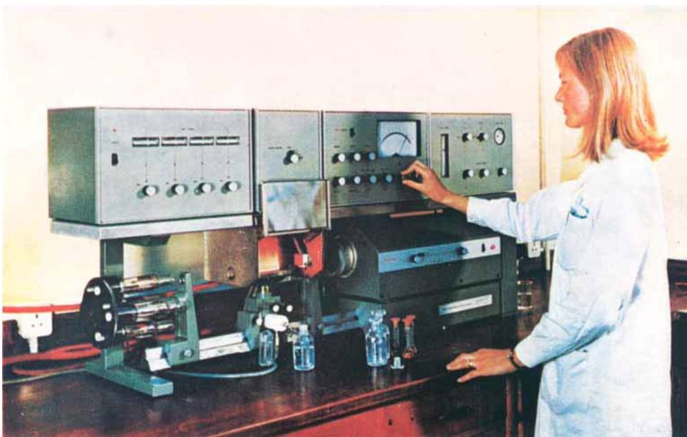
*Atomic absorption spectroscopy is used for the determination of other platinum group metals and of base metals in platinum being processed to check the efficiencies of the separation techniques. It is also used as a rapid check procedure against wet chemical analysis methods and emission spectroscopy*
