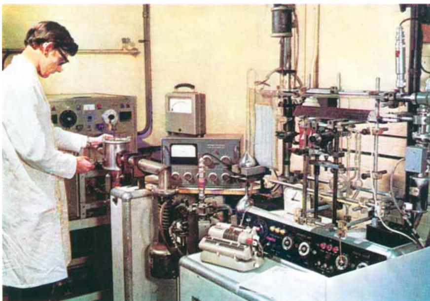
*The determination of oxygen, hydrogen and nitrogen is carried out in the vacuum fusion apparatus. More complete information on the gas content of platinum is obtained in similar equipment where the conventional low pressure gas analyser shown here is replaced by a mass spectrograph*
