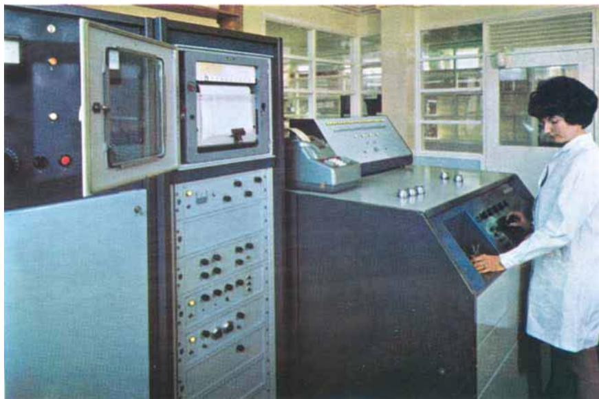
*X-ray fluorescence spectroscopy is used extensively to determine many of the elements in platinum to be refined and for monitoring some stages of the refining operations. This instrument is controlled by a novel logic unit enabling up to 25 elements to be determined automatically. The X-ray data is processed in a central computer*
