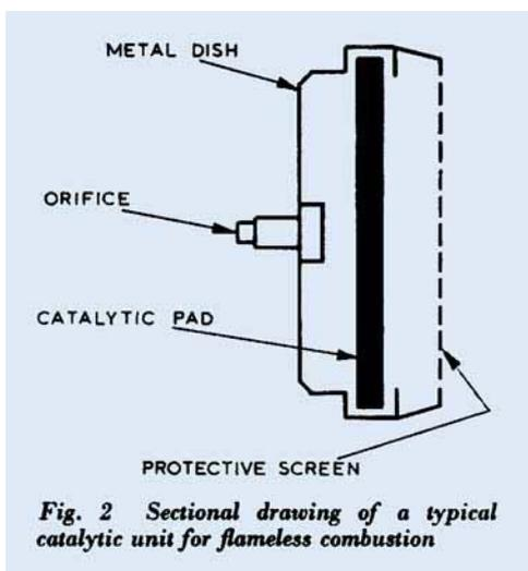
perforated metal screen. The most common shape of catalyst pad (and therefore of heater) is rectangular.
