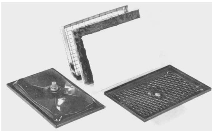
**Fig. 3 Construction of a rectangular propane or methane catalytic heater. In the foreground is the metal plate through which the gas enters and is distributed evenly over the catalyst pad. Left is the back of the plate, showing the gas orifice and right is the inside of the plate. The white pad is a filter pad through which the gas permeates to the catalyst pad, the front face of which is protected by the wire mesh screen**
