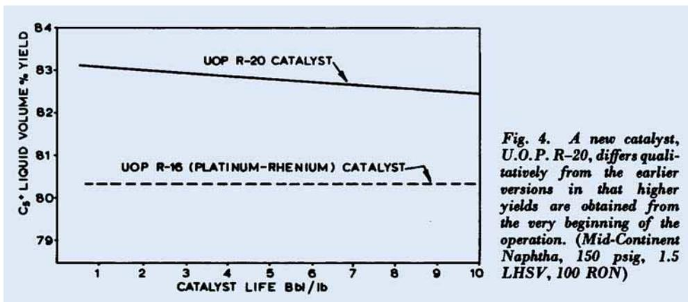
Fig. 4. A new catalyst, U.O.P. R-20, differs qualitatively from the earlier versions in that higher yields are obtained from the very beginning of the operation. (Mid-Continent Naphtha, 150 psig, 1.5 LHSV, 100 RON)
