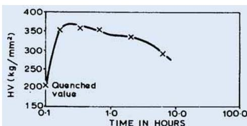
Fig. 2 Order-hardening of stoichiometric copper-platinum alloy; 700°C isotherm
