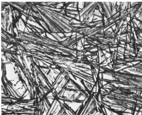
Fig. 3 The microstructure of quenched 70 at.% ruthenium-platinum alloy displays a volumetric distribution of the two phases commensurate with the position of this alloy within the two-phase area
