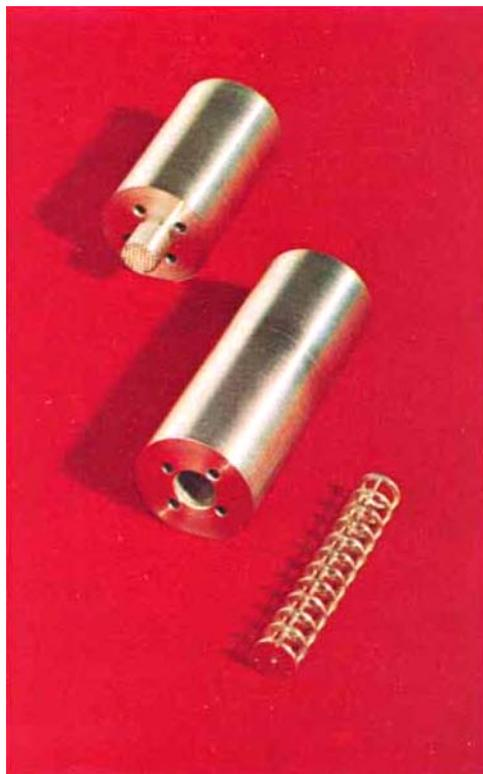
*The three sections forming the black-body cavity consist of a baffle assembly (foreground) with a small hole in its end-plate, a cylinder into which the assembly fits, and a stopper (background) which screws into the latter. The four holes in the cylinder and stopper accommodate the thermocouples under test*
