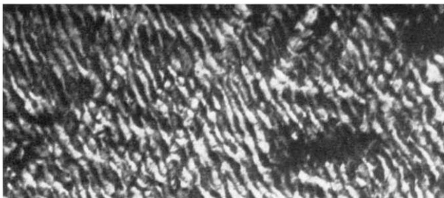
*Fig. 2 Transmission electron micrograph of a thin foil of high coercivity material, reduced to the required thickness by ion bombardment (by M. Paulus of C.N.R.S., Bellevue, France). The fine structure indicated, with 100Å spacing, is assumed to be a consequence of the ordering, although a detailed interpretation is not yet possible.  $\times 50,000$*
