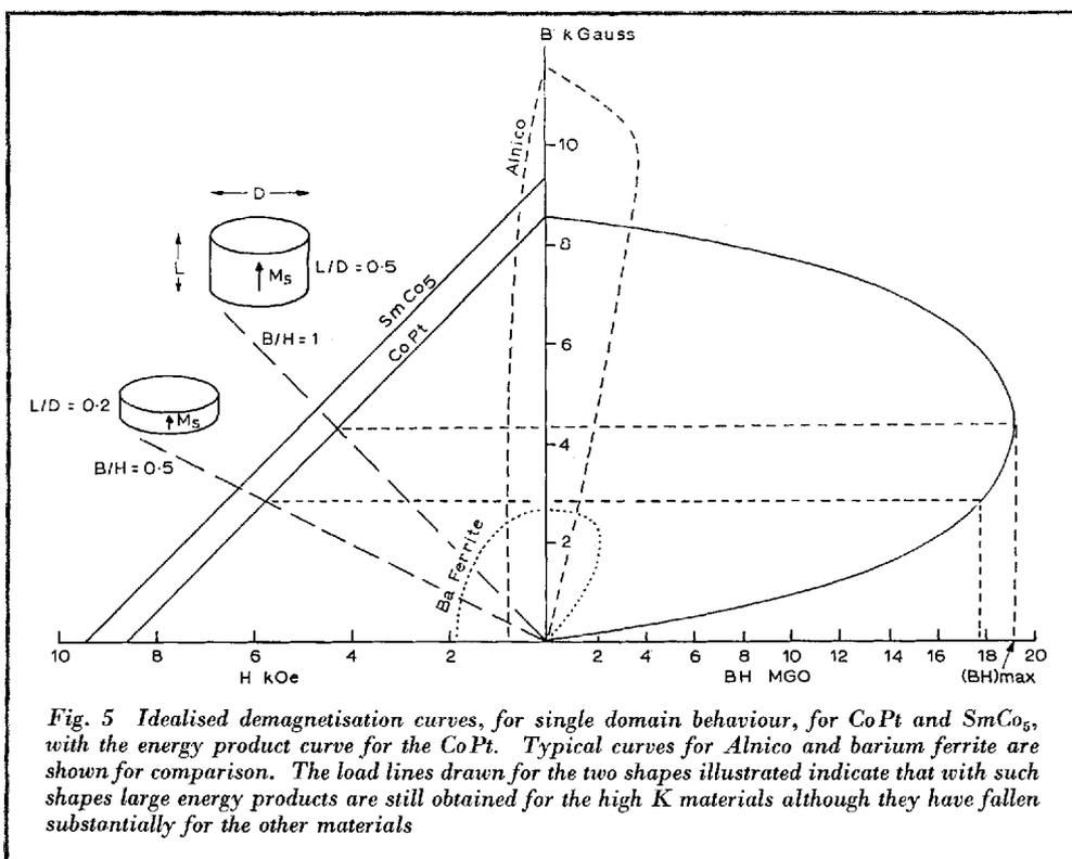
Fig. 5 Idealised demagnetisation curves, for single domain behaviour, for CoPt and SmCo<sub>5</sub>, with the energy product curve for the CoPt. Typical curves for Alnico and barium ferrite are shown for comparison. The load lines drawn for the two shapes illustrated indicate that with such shapes large energy products are still obtained for the high K materials although they have fallen substantially for the other materials
