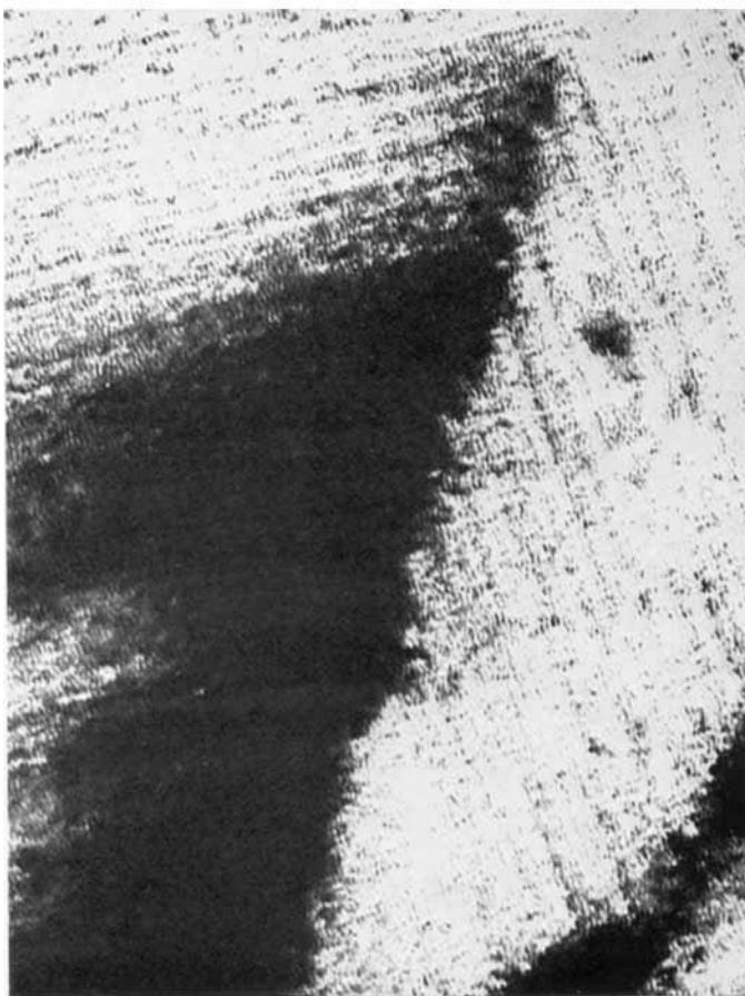
Fig. 3 (b) As (a) at very high magnification, indicating that the striations shown within the domains have themselves an ultra-fine structure with a spacing of about  $100\text{Å}$  which it is tempting to associate directly with the ordering structures shown in Fig. 2.  $\times 32,000$
