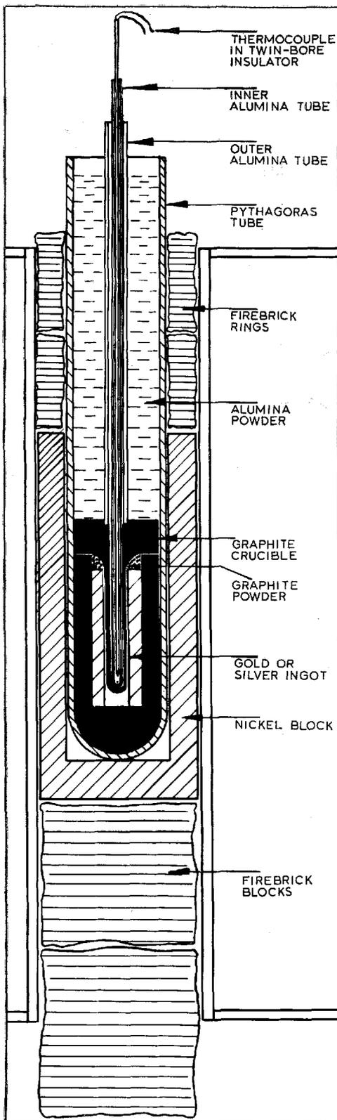
Fig. 2 Section through the N.P.L. apparatus for the calibration of platinum: rhodium-platinum thermocouples at the freezing points of gold and silver
