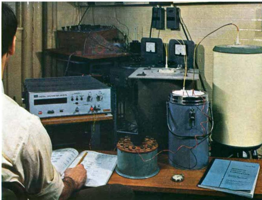
*Fig. 3 Calibration of thermocouples at N.P.L. includes plotting the thermal arrest at the freezing point of silver. The cold junctions are held in the flask of melting ice at 0°C. The use of a reversing switch eliminates the effect of stray e.m.f.s in the measuring system*
