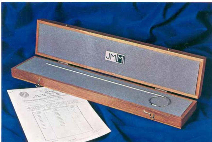
*Fig. 1 A typical Johnson Matthey Metals high accuracy thermocouple in its foam-lined case after calibration at the National Physical Laboratory. With it is its N.P.L. report. The thermocouple is mounted in a one-piece insulator 400 mm long in order to retain its strain-free calibrated condition*
