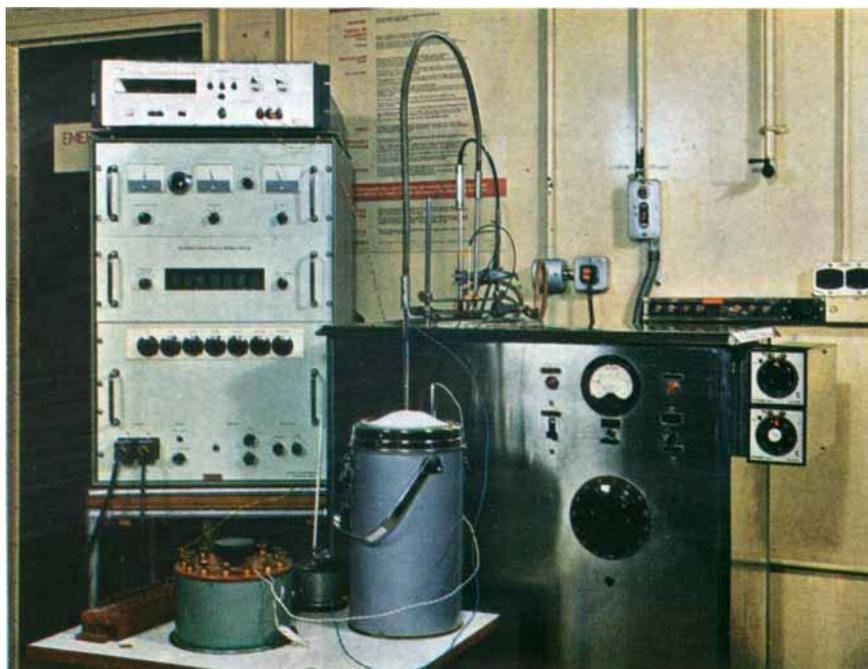
*Fig. 4 Simultaneous comparison at N.P.L. of temperature measurement by means of a platinum resistance thermometer and a.c. double bridge with the thermal e.m.f. of a J.M.M. thermocouple under test in a stirred-liquid salt bath*
