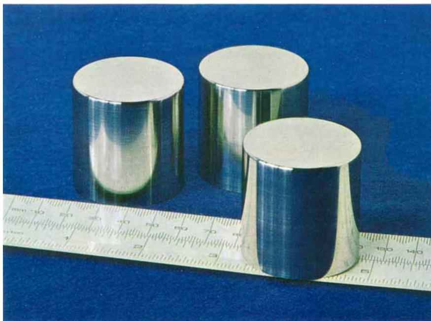
*Fig. 2 A group of three standard 10 per cent iridium-platinum kilograms fabricated by Johnson Matthey Metals for the Bureau International des Poids et Mesures. The purity of the alloy and the dimensions and density of the cylinders are controlled to a rigorous specification. Diameter is made 39.2 mm, height 39.5 mm and density 21.53 g/cm<sup>3</sup>*
