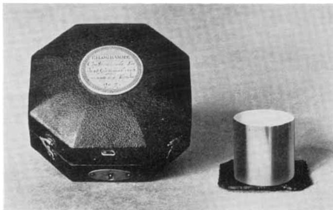
*Fig. 1 This standard kilogram was made by Janety using platinum. The label on the case states “Kilogramme Conforme ala Loi du 18 Germinal An 3 [April 7th, 1795], présenté le 4 Messidor An 7” [June 23rd, 1799]*
