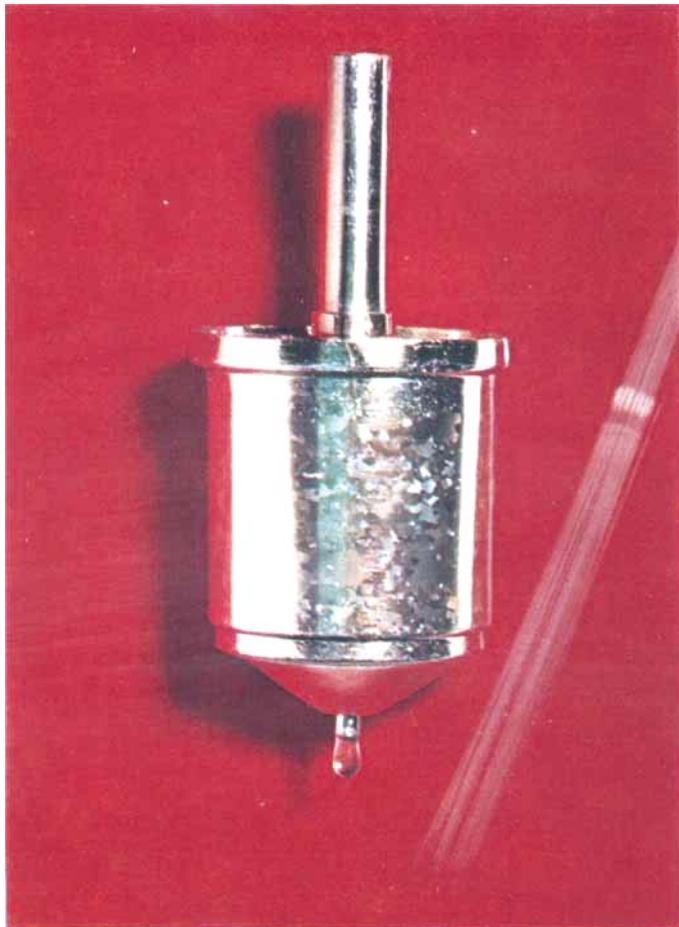
*This bushing for the production of optical glass fibres, some of which are illustrated, is fabricated from the new high purity Fibre Optic grade of platinum*
