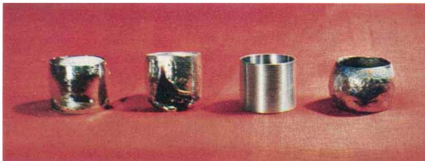
*Fig. 3 New and used crucibles of 30 cm<sup>3</sup> capacity. From the left are shown: a crucible slightly distorted by yttrium aluminium garnet; a crucible which has failed by melting; a new crucible made from welded sheet; a crucible heavily distorted and oxidised by gadolinium gallium garnet*
