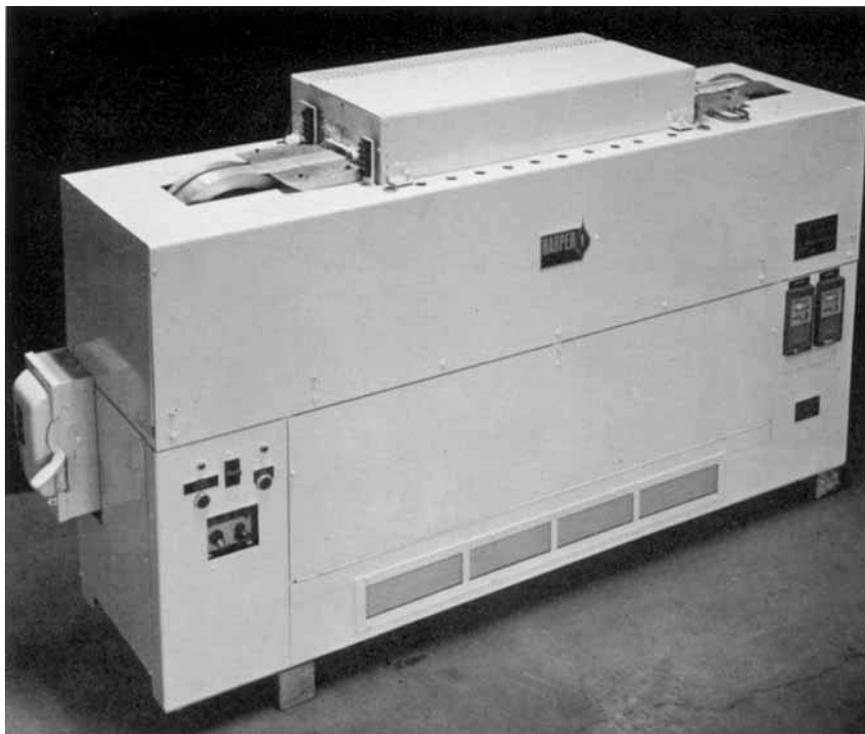
*A Harper electric furnace for sintering ferrite cores. The platinum alloy belt can be seen passing over the pulleys at each end of the furnace section. The belt is made endless by weaving the warp wires or by hammer welding*
