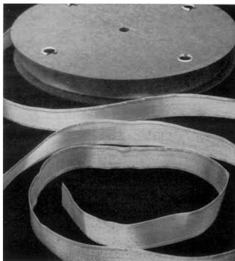
*A reel with a belt of rhodium-platinum gauze produced by Matthey Bishop Inc. Belts up to 5 inches wide are made. Belt length depends upon furnace dimensions. The gauze can withstand the process temperature of up to 1500°C without deformation, core contamination or core adherence*
