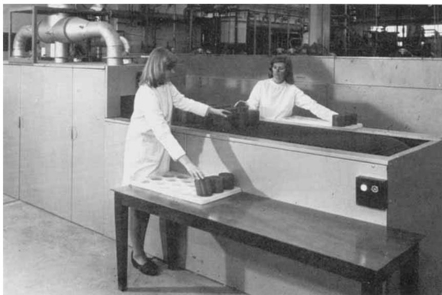
*Finished honeycomb catalyst pieces being removed from the furnace conveyor belt after firing at the Royston factory of Johnson Matthey Chemicals Ltd. They will be incorporated in automobile catalyst systems by European manufacturers of motor vehicles*
