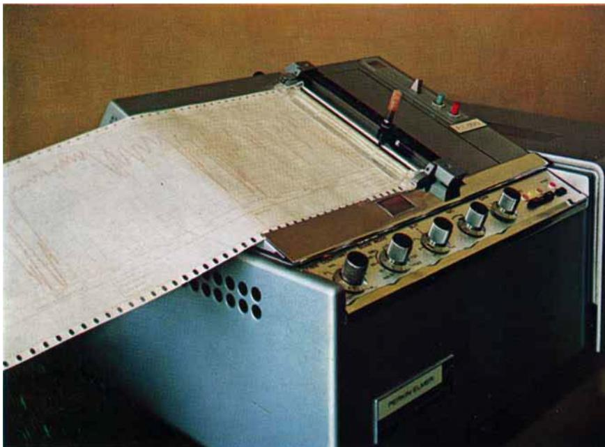
*A wide range (4000 to 200  $\text{cm}^{-1}$ ) infra-red spectrophotometer used to characterise platinum group metal coordination complexes. The low frequency region (600 to 200 $\text{cm}^{-1}$ ) is particularly useful for this type of compound*
