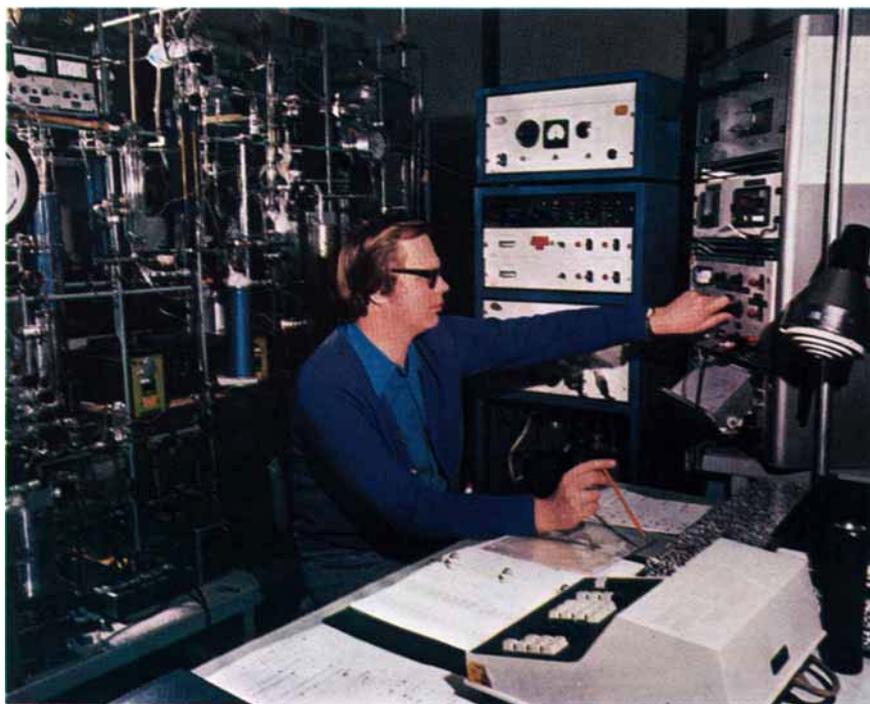
*Fig. 1 Research workers at Atomic Energy of Canada Limited have found that the mass spectrometer is an indispensable tool for the study of isotopic exchange reactions. This instrument monitors the deuterium content of hydrogen from the catalytic reactor*
