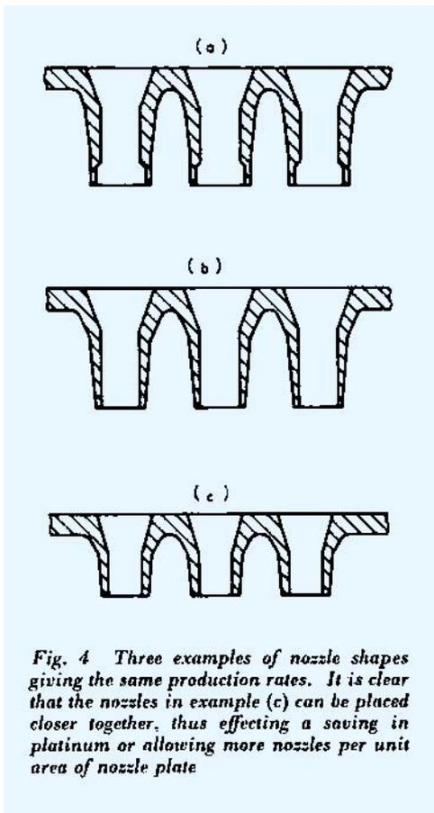
*Fig. 4 Three examples of nozzle shapes giving the same production rates. It is clear that the nozzles in example (c) can be placed closer together, thus effecting a saving in platinum or allowing more nozzles per unit area of nozzle plate*
