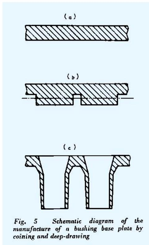
*Fig. 5 Schematic diagram of the manufacture of a bushing base plate by coining and deep-drawing*
