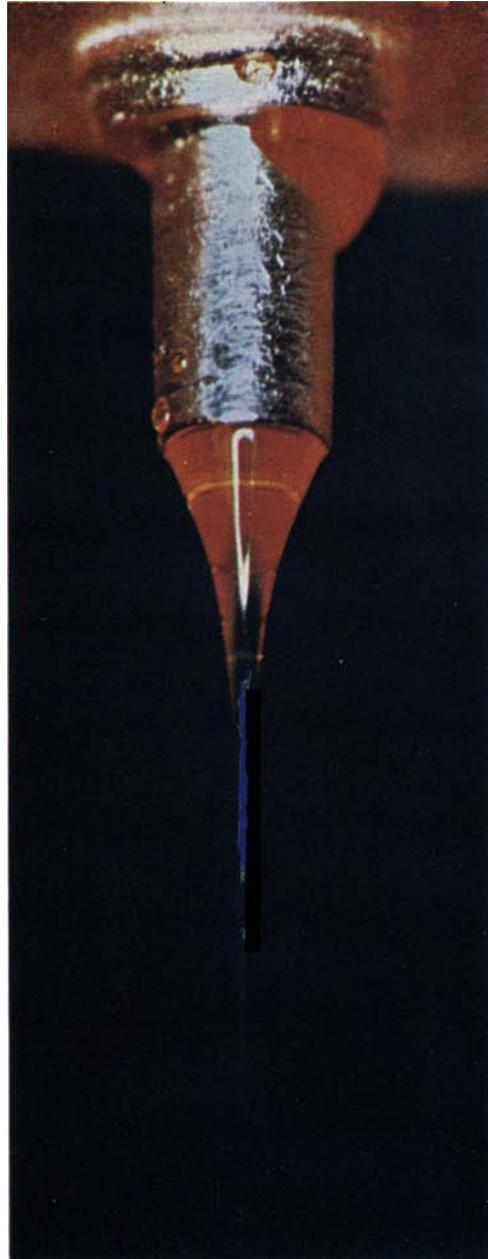
*Fig. 1 Glass-fibre filaments are formed by drawing molten glass through hundreds of small orifices in a bushing constructed in a rhodium-platinum alloy. Great attention is given to the design of the bushing and to the method of manufacture of the nozzles to achieve maximum productivity. At the very high temperatures at which the process is operated only platinum alloys possess the necessary strength, while their use is most economical in terms of the amount of fibre produced.*
