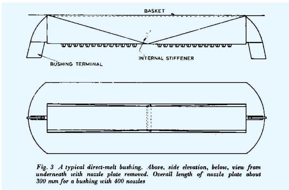
Fig. 3 A typical direct-melt bushing. Above, side elevation, below, view from underneath with nozzle plate removed. Overall length of nozzle plate about 300 mm for a bushing with 400 nozzles
