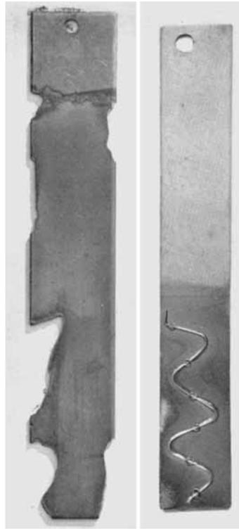
*Fig. 2 (left)—Severe corrosion of titanium anode after operation for a short time in sea-water at a current density of 24 amp. per square foot*
