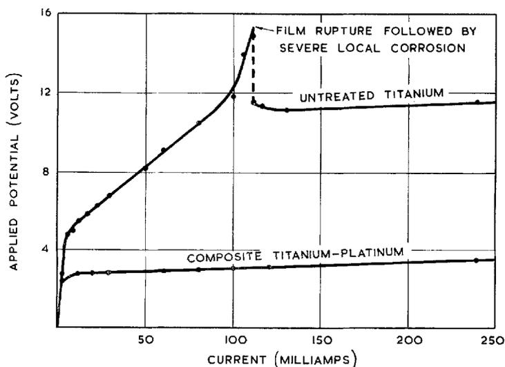
Fig. 1 Current-voltage characteristics of untreated titanium and of composite titanium-platinum in sea-water
