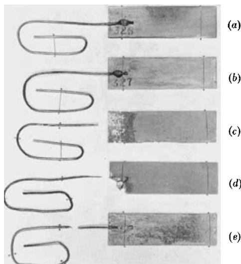
Fig. 5 Specimens of titanium coated with approximately 0.000005 inch of platinum after operation at an anodic current density of 60 amp. per square foot in sea-water at room temperature
