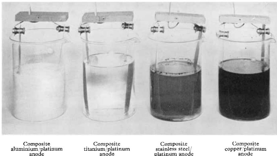
*Fig. 4 The unique property of titanium is demonstrated in this illustration, which shows beakers of sea-water containing composite anodes after four hours' service at an overall current density of 24 amp. per square foot. A titanium cathode was used in each beaker*
