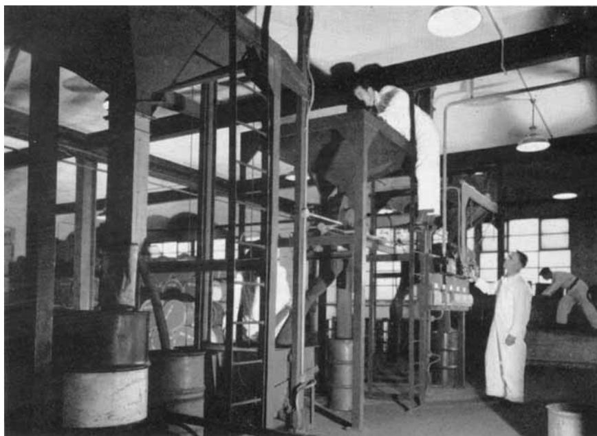
*The sampling plant in the Johnson Matthey refineries, specially designed for handling spent reforming catalyst*
