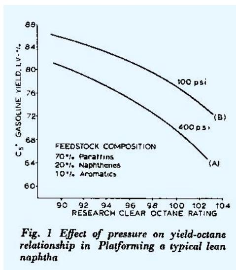
**Fig. 1 Effect of pressure on yield-octane relationship in Platforming a typical lean naphtha**
