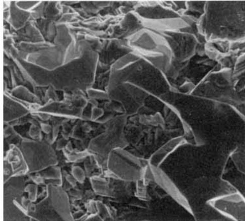
*Fig. 23 Front of gauze 2 used in a medium pressure plant, secondary electron image*  $\times 2000$
