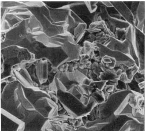
*Fig. 25 Front of gauze 3 used in a medium pressure plant, secondary electron image*  $\times 2000$
