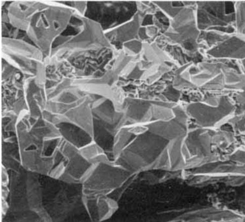
*Fig. 22 Rear of gauze 1 used in a medium pressure plant, secondary electron image*  $\times 2000$
