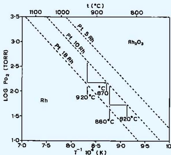
Fig. 20 Temperature dependence of oxygen partial pressure for formation of rhodium oxide on rhodium-platinum alloys
