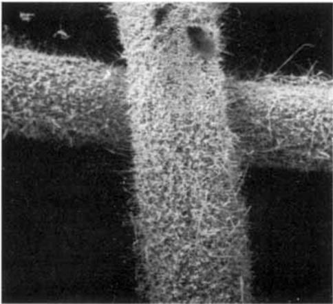
*Fig. 16 Front of gauze 3 used in a medium pressure plant*  $\times 200$
