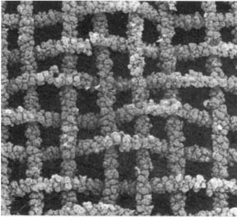
*Fig. 13 Front of gauze 1, atmospheric pressure plant, secondary electron image*  $\times 44$
