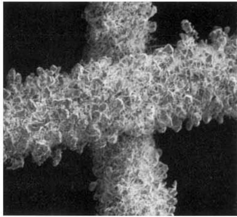
*Fig. 14 Front of gauze 2 used in a medium pressure plant*  $\times 200$
