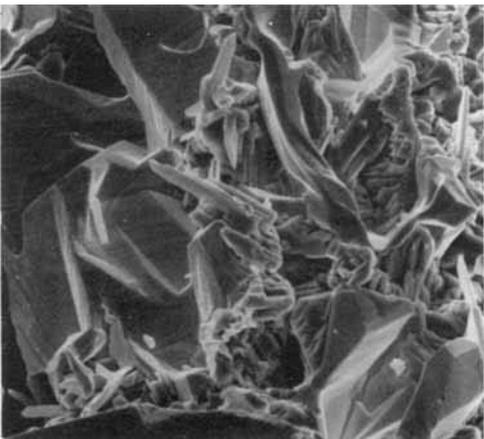
*Fig. 24 Rear of gauze 2 used in a medium pressure plant, secondary electron image*  $\times 2000$
