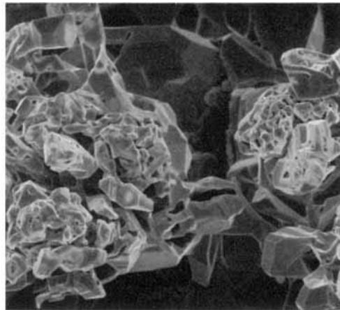
*Fig. 21 Front of gauze 1 used in a medium pressure plant, secondary electron image*  $\times 2000$
