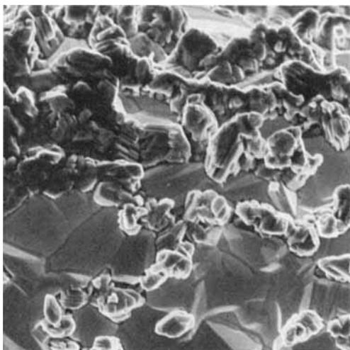
Fig. 26 Rear of gauze 3 used in a medium pressure plant, secondary electron image  $\times 2000$
