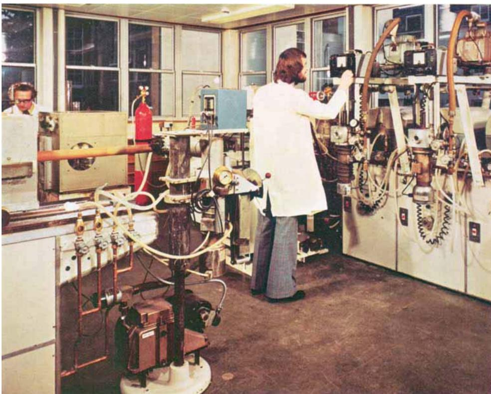
*Comprehensive facilities are available for studying many aspects of the platinum group metals, for which increasing applications are continually being found in the advanced technology industries. In the furnace room, shown above, the unique high temperature properties can be investigated under a controlled atmosphere or in vacuum*
