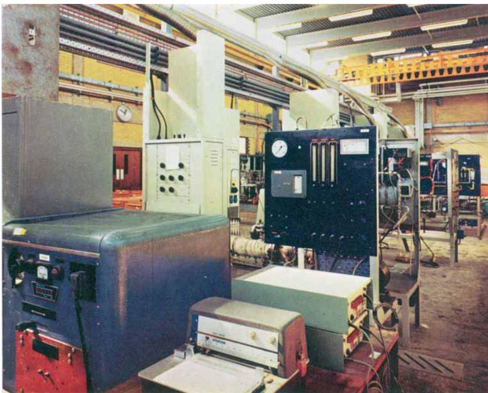
*A large project area suitable for pilot plant development, or readily adaptable to changing research requirements, is provided in one of the blocks. The equipment in this area, part of which is shown above, includes a number of test rigs used for the continuing investigation and evaluation of catalytic units for automobile emission control*
