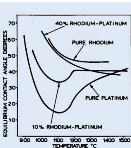
Fig. 2 The equilibrium contact angle of 'E' glass on pure platinum and rhodium-platinum alloys as a function of temperature
