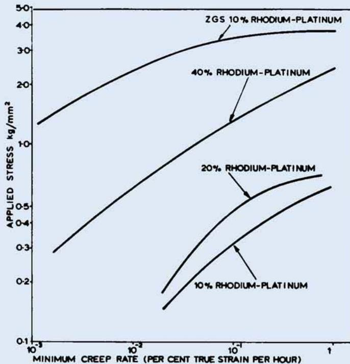
Fig. 6 Minimum creep rate curves for ZGS 10 per cent rhodium-platinum and the commonly used rhodium-platinum alloys in sheet form, tested at 1400°C in air
