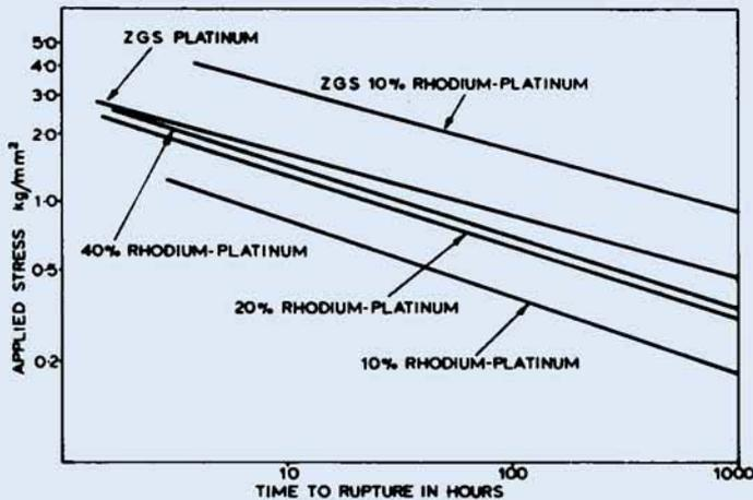
Fig. 5 Stress rupture properties of ZGS platinum, ZGS 10 per cent rhodium-platinum and the commercially important conventional alloy compositions. The curves refer to tests carried out at 1400°C in air on 1.5 mm thick sheet specimens
