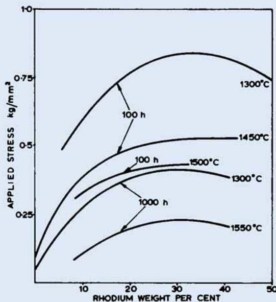
**Fig. 1 Stress rupture data for rhodium-platinum alloys of varying rhodium content (2)**
