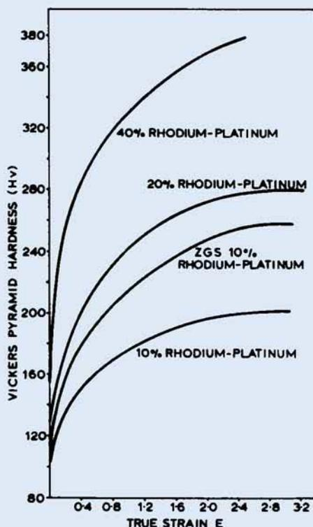
Fig. 3 Work-hardening characteristics of ZGS 10 per cent rhodium-platinum compared to those of the traditional melted alloys
