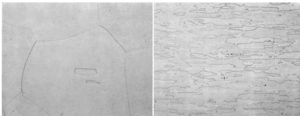
Fig. 4 The microstructures of 10 per cent rhodium-platinum (left) and ZGS 10 per cent rhodium-platinum (right) after heating for 500 hours at 1400°C in air. The high stability of the oxide-stabilised alloy is well illustrated by these photomicrographs × 50
