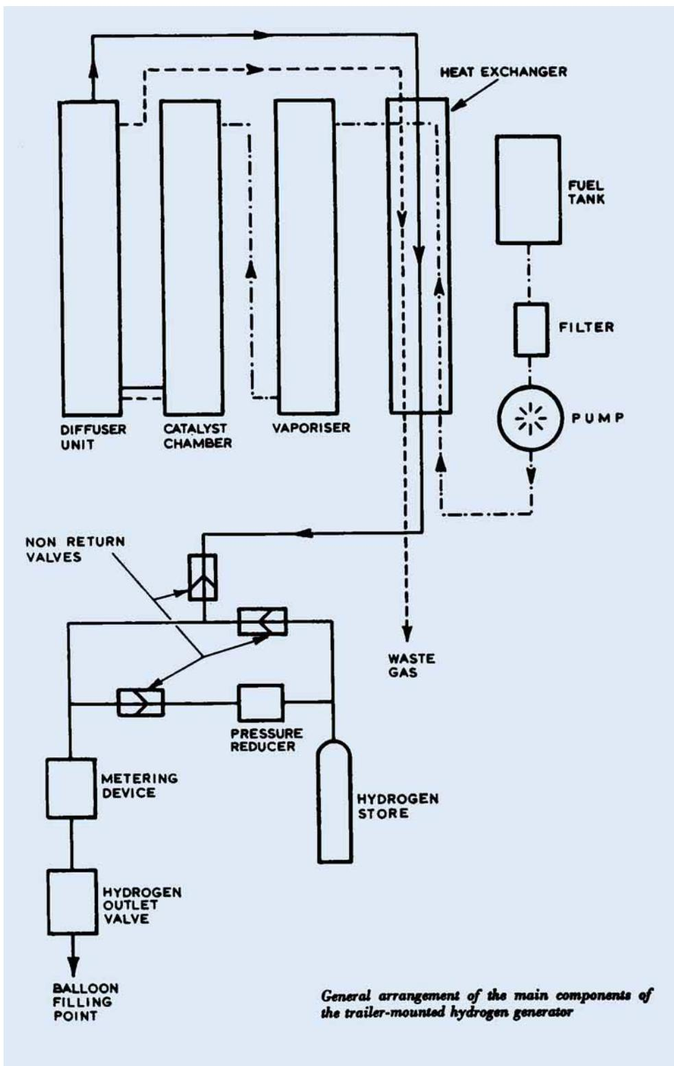
During production the fuel, a 1 : 1 molar methanol/water mixture, is pumped through a heat exchanger then into a vaporiser, as shown in the Figure opposite, before entering the catalyst chamber where the methanol is cracked into hydrogen and carbon monoxide. Subsequently steam reacts with the carbon monoxide to produce carbon dioxide and more hydrogen all of which passes into the diffusion module.
