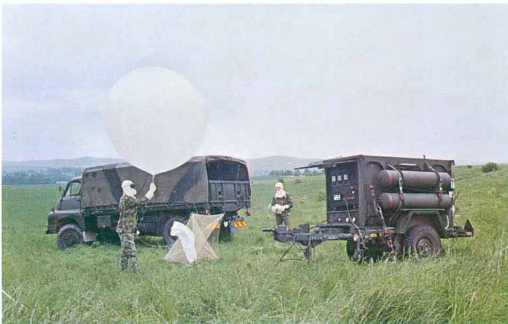
*A hydrogen generator undergoing field trials with the British Army. The balloon which is about to lift the radiosonde equipment into the atmosphere, has just been inflated with pure, dry hydrogen produced on-site. As the generation of hydrogen proceeds the gas is used to fill the hydrogen storage cylinders in readiness for the next launch*
