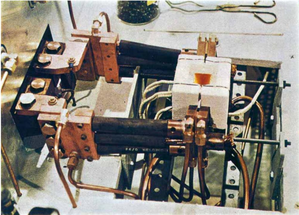
*Fig. 3 In the experimental set-up for basalt fibre forming the bushing is insulated with a high purity porous refractory. Heavy, flexible, water-cooled conductors connect the power supply to the bushing while the fibre blowing nozzle and fibre winding drum are located below the bushing*
