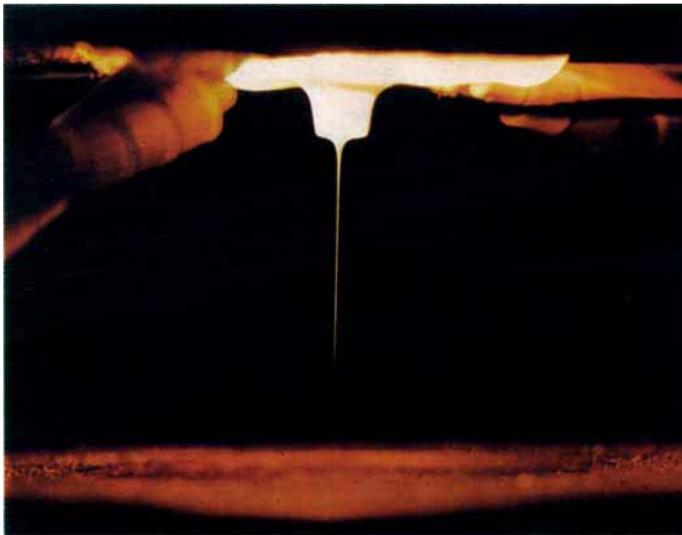
*Fig. 4 Basalt fibre being drawn from the bushing orifice. Fibres having a wide size range can be produced in the laboratory by varying the speed of drawing and the temperature of the melt*
