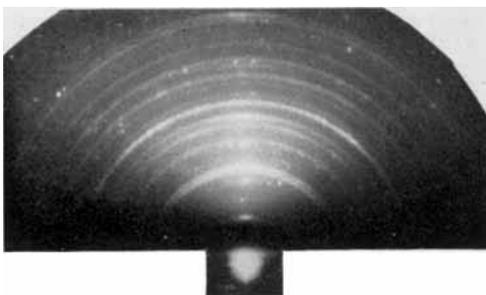
Fig. 2 Electron diffraction pattern from the platinum-10 weight per cent palladium alloy. The reflections correspond to an intermetallic compound with a superlattice structure whose long period is 86.5 Å, and is presumed to be Pt<sub>3</sub>Pd
