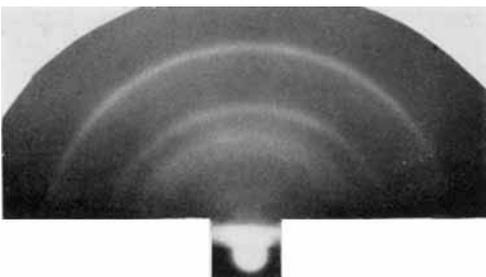
Fig. 3 Diffraction pattern of the platinum-palladium on alumina paste prepared from the alloy illustrated in Figure 2. This pattern is similar to that shown in Figure 1
