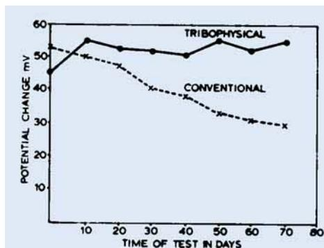
**Fig. 5** The catalytic life of material produced by the tribophysical method, shown by the solid line, compared with that of conventionally produced material, broken line, by means of the potential change shown by the recorder when the catalytic activity is taking place. Apart from the initial period, the tribophysical material is superior
