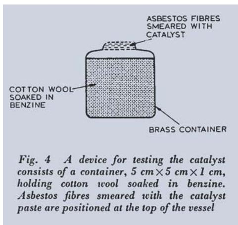
Fig. 4 A device for testing the catalyst consists of a container, 5 cm × 5 cm × 1 cm, holding cotton wool soaked in benzene. Asbestos fibres smeared with the catalyst paste are positioned at the top of the vessel
