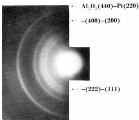
*Fig. 1 Electron diffraction pattern obtained from the paste produced when a platinum plate was mechanically polished with gamma-alumina abrasive. This pattern verifies the presence of particles of uniform size, estimated to be about 50 Å.*
