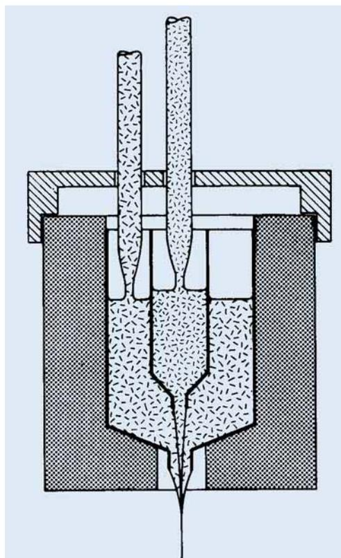
*The double platinum crucible for the production of optical glass fibres. The inner rod of alkali-germanosilicate glass has a high Na<sup>+</sup> ion content and a high refractive index, while the outer rod of the same glass but with a high K<sup>+</sup> ion content has a low refractive index. Between the outlets of the concentric crucibles there is an exchange between the Na<sup>+</sup> and the K<sup>+</sup> ions, giving a smooth variation of the refractive index profile in the resulting fibre*
