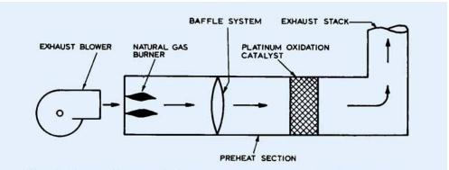
Schematic diagram illustrating the flow of gas through the unit. The polluted process gas is heated to the required temperature, passed through the stainless steel baffles and purified by the platinum catalyst, after which harmless carbon dioxide and water are discharged
