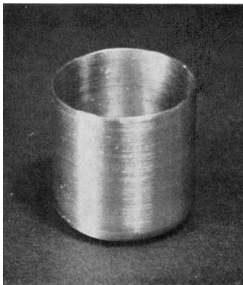
Fig. 7 This platinum crucible, shown here approximately twice full size, was produced by an electro-forming process
