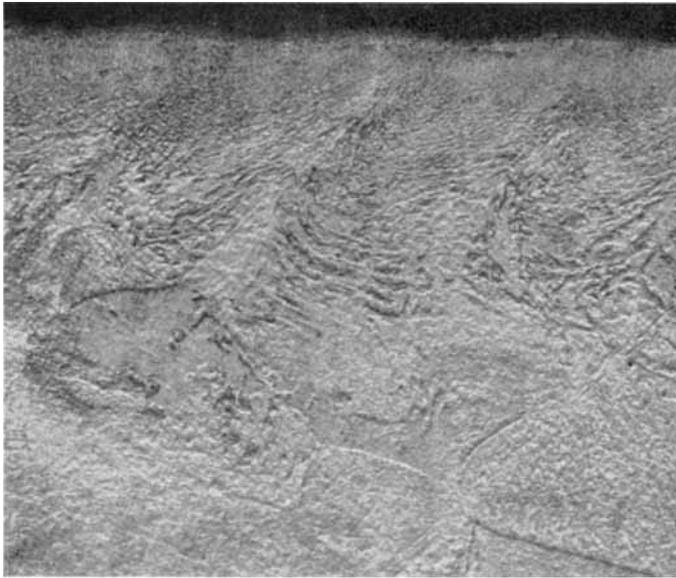
*Fig. 7 The surface deformation which occurred when an annealed platinum bar was machined with a progressively wearing tungsten carbide tool. Even a single cut with a sharp tool introduces a high degree of strain into the surface of the platinum and results in a large increase in hardness*
