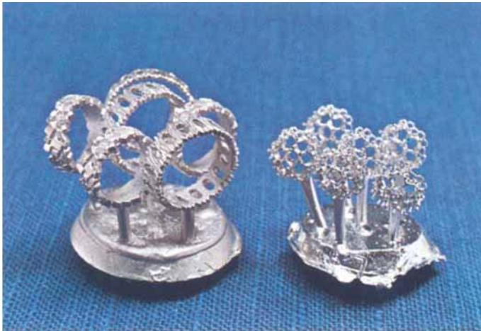
*Fig. 2 Two typical platinum buttons show the limited number of well-spaced items that can be satisfactorily cast at the elevated temperatures involved*
