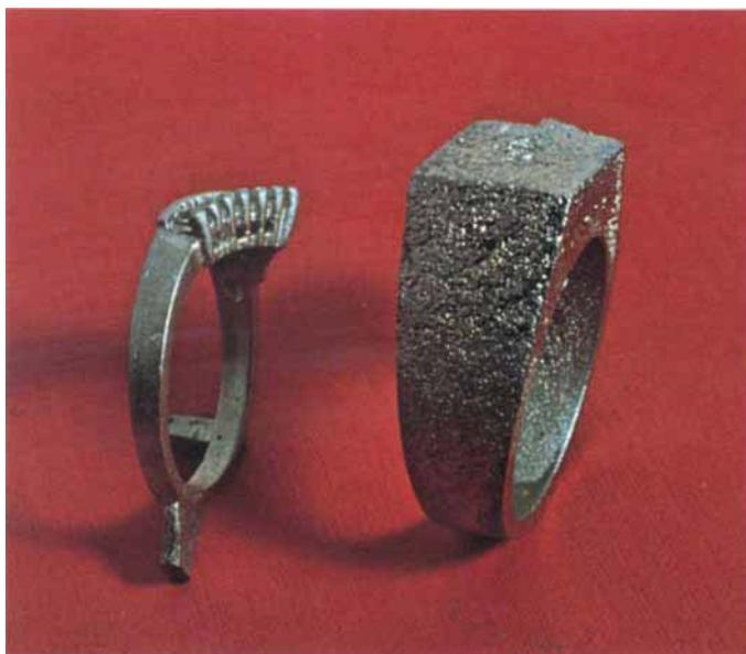
*Fig. 3 The surface erosion, seen on the heavier sectioned ring cast in 4.5 ruthenium-platinum, results from breakdown of the investment. On the lighter sectioned ring this reaction is minimal*
