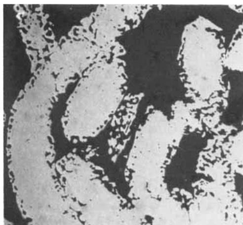
*Fig. 5 A section through the trailing gauze of the pack shows the wire to consist of a solid core surrounded by a porous layer* ×140
