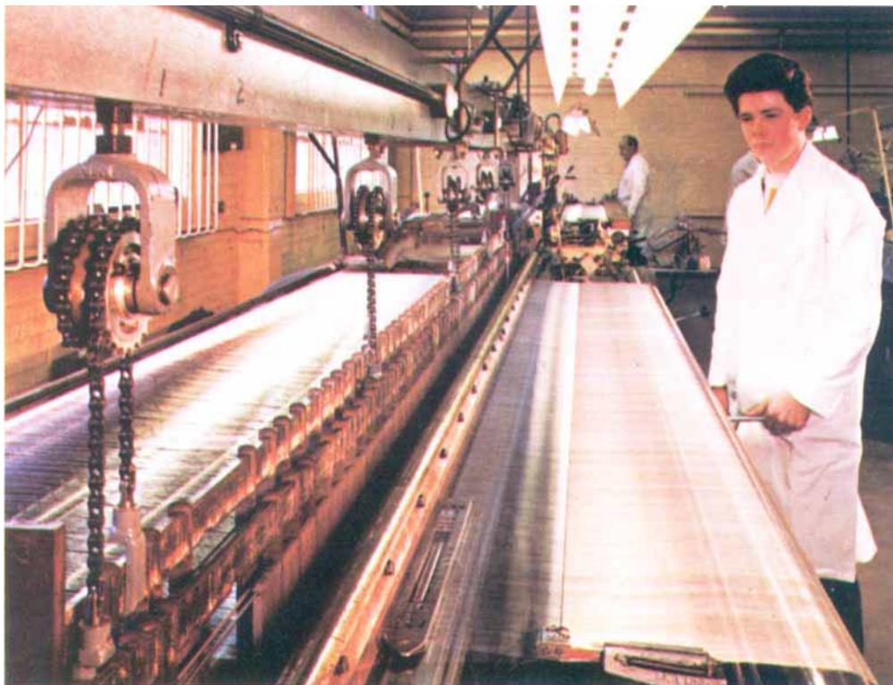
*Fig. 1 Because of its great resistance to oxidation at high temperatures, in addition to its high catalytic activity, platinum—in the form of rhodium-platinum gauze here seen being woven—is employed in the production of nitric acid by the oxidation of ammonia, a process operating at around 850°C*
